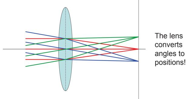
Parallel rays are focused onto the focal plane: in the limit  $u \rightarrow \infty$  then  $v \rightarrow f$
