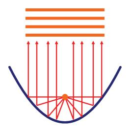
Place a source as indicated at the "focus" of the mirror. This will produce plane wavefronts if the red lines all have the same length
