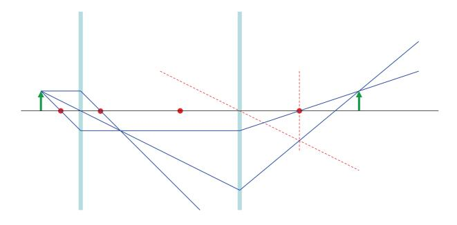
Can ray trace in complex systems by constructing "assistant rays" parallel to the ray of interest and passing through the centre of a lens
