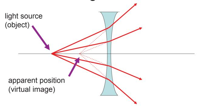
Virtual images of extended objects are scaled down by v/u and upright (draw a ray diagram to check)
