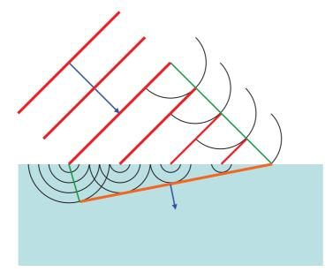
The two green lines are both four wavelets long. The start points of each line are points on a wavefront and so the end points must also be corresponding points on the new wavefront
