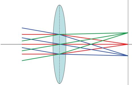
Parallel rays are focused onto the focal plane: in the limit  $u \rightarrow \infty$  then  $v \rightarrow f$
