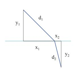
$$t = \frac{d_1}{v_1} + \frac{d_2}{v_2} = \frac{n_1 d_1}{c} + \frac{n_2 d_2}{c}$$
