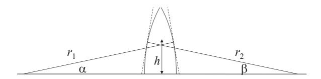
A lens is formed by a pair of curved surfaces. The angle of the equivalent prism is the angle between the surface tangents, which equals the sum of  $\alpha$  and  $\beta$ .
