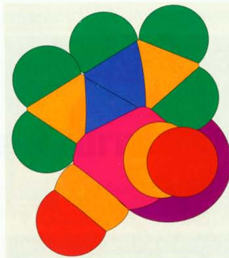
1 This perfluorobutadienyl iron complex is used as a system of seven qubits. The large purple sphere represents a cyclopentadienyl ( C_5H_5 ) ring. The seven nuclei used were the five naturally occurring fluorine-19 nuclei (green) and the two specifically labelled carbon-13 nuclei (blue). The remaining atoms simply form a structural framework and play no part in the computation.
