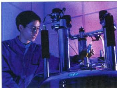
Compute this – Isaac Chuang loads the vial containing the seven-qubit quantum-computer molecules into the NMR apparatus.
