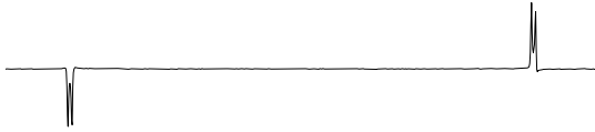
Fig. 1. NMR spectrum showing readout from a two qubit NMR quantum computer based on the two ^1\text{H} nuclei in cytosine [33]; the negative intensity on the left hand multiplet indicates that the corresponding qubit was in state |1\rangle , while the positive intensity indicates that this qubit was in state |0\rangle .
