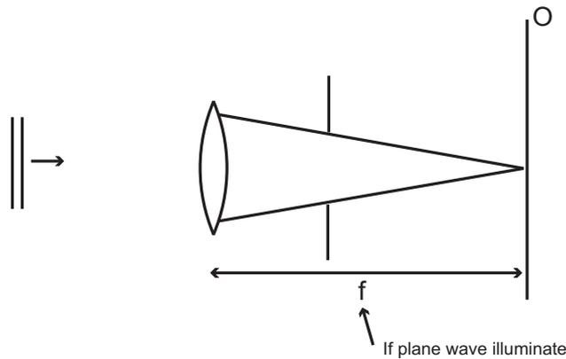
The observation plane is located at the source image. The field at this plane is an exact Fourier Transform of the field at the aperture.
