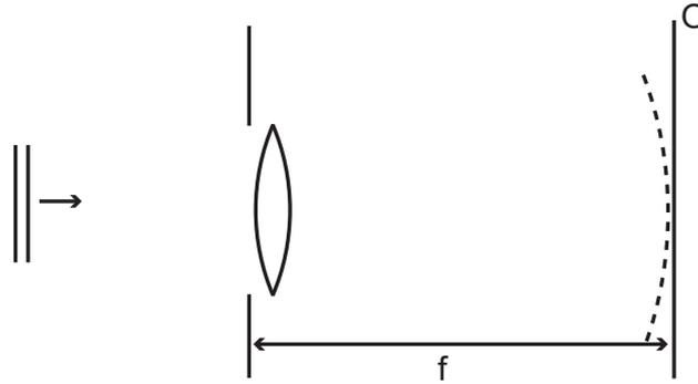
3. Lens before aperture - plane or diverging illumination at the lens
