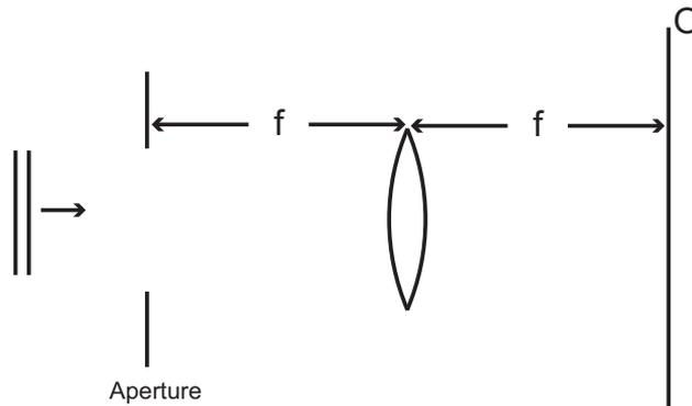
The field at  $O$  is an exact Fourier transform of the aperture function, with no extraneous phases, provided the aperture is illuminated with plane waves. This example will be explored in the homework
