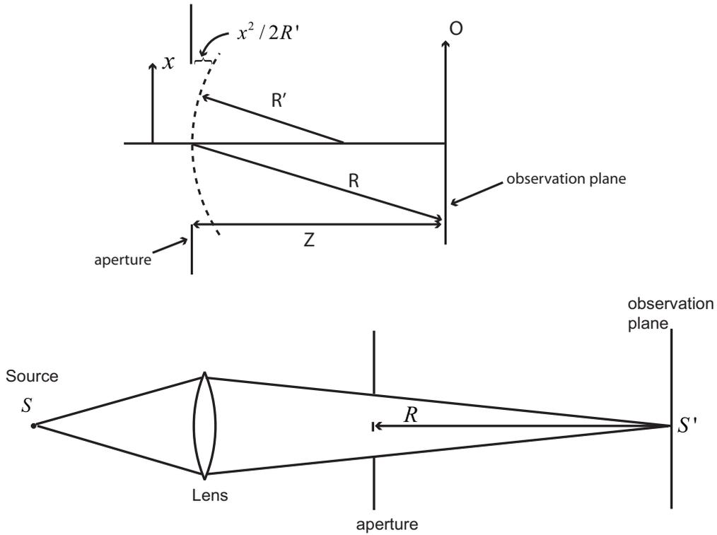
This time the Fourier Transform is exact, and there are no extraneous field-angle dependent phase terms. But how do we set up this configuration? Simple, we need a converging beam on the aperture, so we use a lens.
