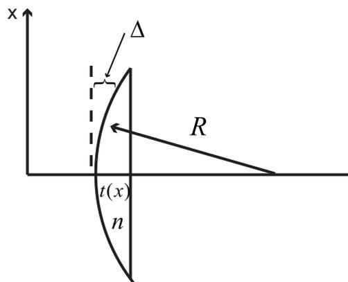
The phase  $\xi(x)$  at position  $x$  accumulated by a plane wave incident from the left of this lens is
