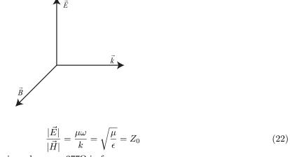
$Z_0 = \text{ impedance } = 377\Omega \text{ in free space}$
