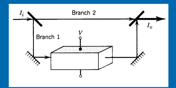
Mach-Zehnder interferometer with a phase modulator in one arm
