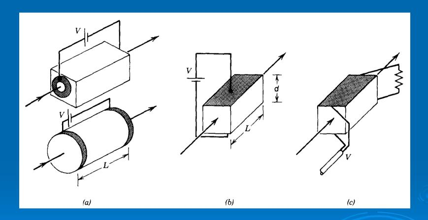
(a) Longitudinal field; (b) Transverse field; (c) Travelling-wave field.
