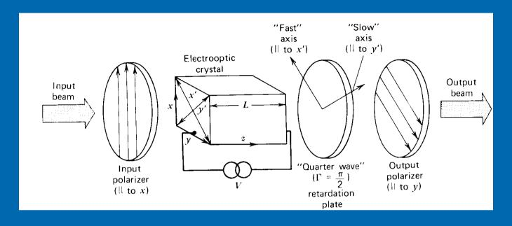
Inserting a quarter-wave plate provides a static bias to point *B* providing a near linear response
