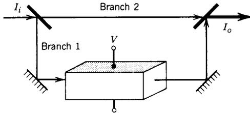
Principle of the Mach-Zehnder Interferometer
