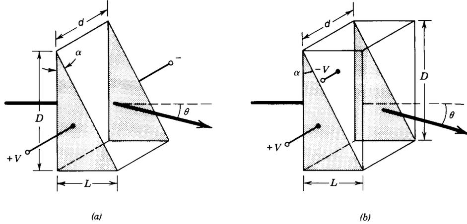
Figure 3: Electro-optic deflection of light.
