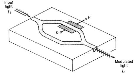
Optical fibre version of a Mach-Zehnder
