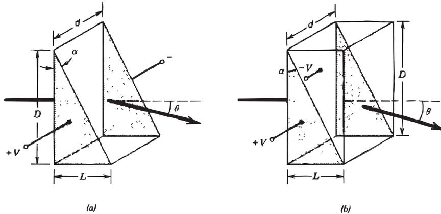
An electric field reversed with respect to the first then doubles the electro-optic deflection while canceling the static crystallographic deflection.
