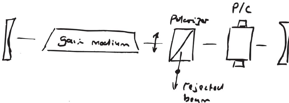
With a voltage applied to the Pockels cell it acts as a quarter-wave plate and hence the combination of linear polarizer and Pockels cell rejects the oscillating modes. However if this voltage is removed the Pockels cell does not change the polarization state of the mode and hence the cavity losses are reduced. [Other possible approaches include acousto-optic modulation, Kerr lens mode locking, the use of a saturable absorber, frequency modulation with a Pockels cell or an AOM.]
