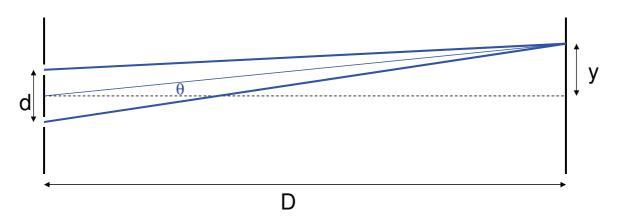
As y<<D the three blue lines are effectively parallel and all make an angle  $\theta \approx y/D$  to the normal. The bottom line is slightly longer than the top.
