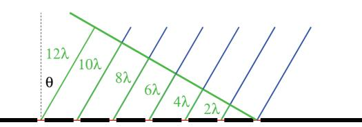
Can also get diffraction in the same direction if the wavelength is halved!
