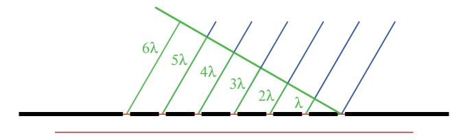
Points on a wavefront must be in phase, so the extra distances travelled must be multiples of a wavelength
