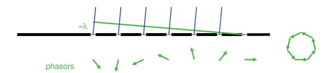
With an *finite* number of sources the last effective cancellation will occur when the path length difference between the first and last sources is about  $\lambda$
