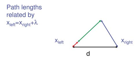
Next line is locus of points where distance from the two slits differs by one wavelength
