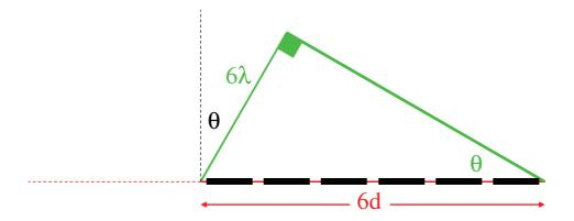
From trigonometry we see that  $\sin(\theta)=6\lambda/6d$  where  $\theta$  is the angle between the ray direction and the normal
