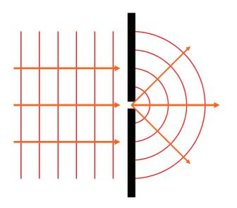
A plane wave impinging on a *infinitesimal* slit in a plate.
