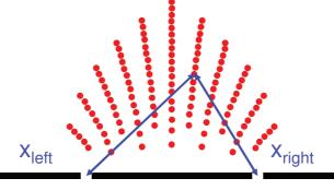
Next line is locus of points where distance from the two slits differs by one wavelength
